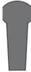
Small Falling Target 20 cm diameter with 1cm cut on both sides with 18cm width at sides at widest point 56 cm height
