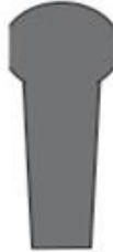
Small Falling Target 20 cm diameter with 1cm cut on both sides with 18cm width at sides at widest point 56 cm height
